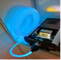
Stranded side glow fiber optic light cable is a multistring fiber which can transmit light over reasonably long distances. Light is transmitted over the entire length of the cable without electricity or heat. The light engine is an illuminator which is placed at one or both ends of the fiber cable.
